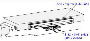
N Do not tighten prior to adjusting leveling set screws
