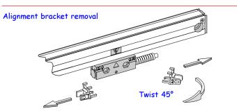
Slide brackets away from reading head and cable.
