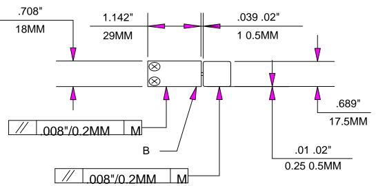
M = MACHINE GUIDEWAY B = MOUNTING SURFACE
