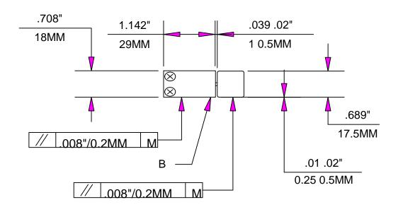
M = MACHINE GUIDEWAY B = MOUNTING SURFACE
